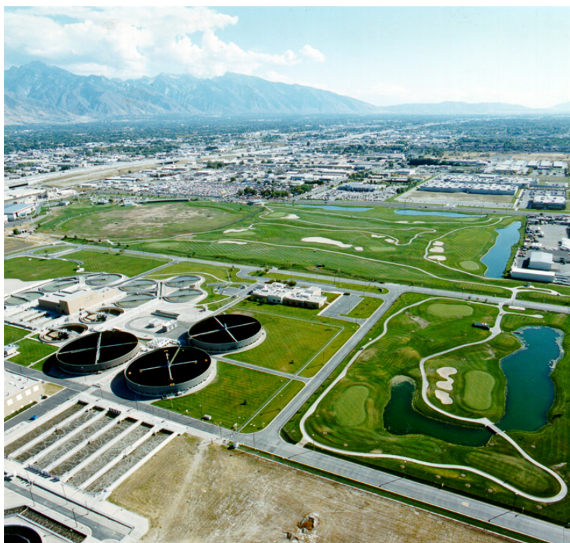
The Central Valley Golf Course receives approximately 0.6 million gallons per day of reclaimed water from the Central Valley Water Reclamation Facility to irrigate its greens and fill the various decorative ponds. (Photo courtesy of Central Valley Water Reclamation Facility.)
