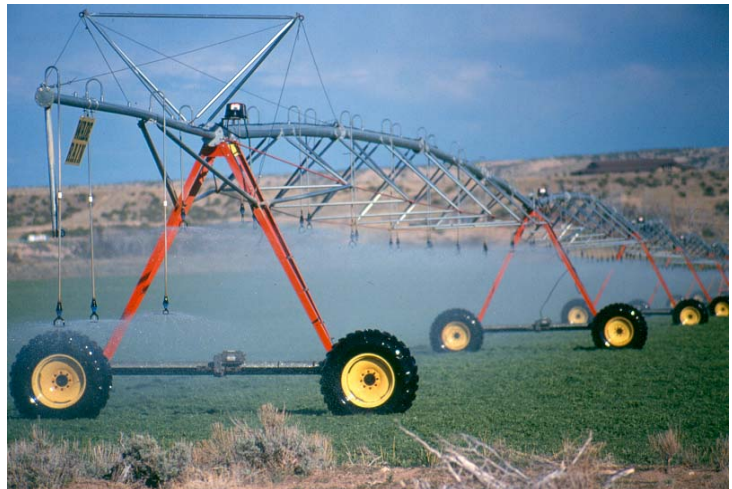
Sprinkler irrigation is only allowed with Type II effluent if there is a buffer of 300 feet or more from public access and potable wells.
