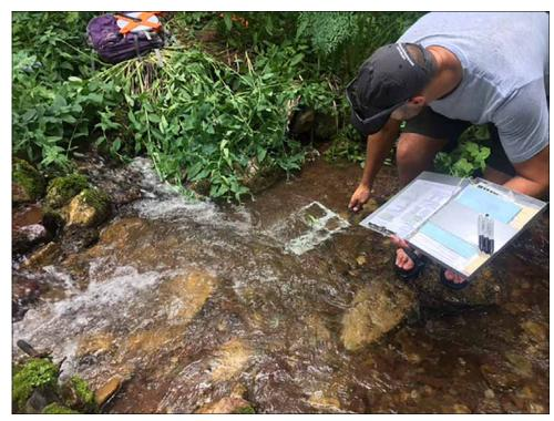
A device called a "gravelometer" (shown in the water) is used to measure the size of sediments (pebbles, cobbles, etc.) found in the stream banks and bed. This is one of many data variables collected by the Watershed Program to assess stream channel stability.
